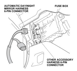
18. Secure the automatic day/night mirror harness to the vehicle harness with two wire ties.
