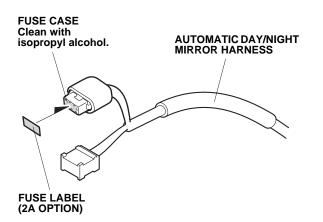
15. Attach the fuse label to the automatic day/night mirror harness fuse case.
